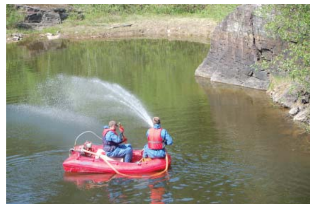
Fig. 2 Boat mounted pump used to apply BETAMAX VET® during the Dammane and Ostøya treatments.
